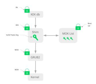
FIGURE 11.2: UEFI: SECURE BOOT PROCESS
