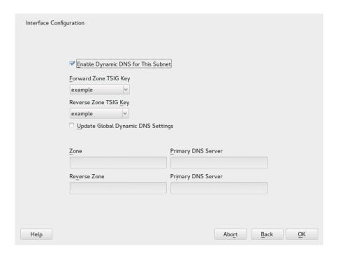
FIGURE 27.10: DHCP SERVER: INTERFACE CONFIGURATION FOR DYNAMIC DNS
